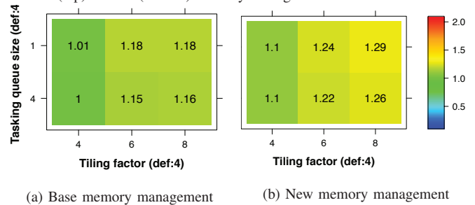
(a) Base memory management (b) New memory management Fig. 10. Performance improvement with space exploration using multiple tiling factors and scheduling quanta (P3 on Carver using 32 threads).
