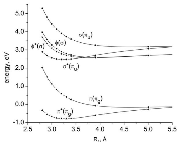
FIG. 9. Potential energy profiles along interfragment separation in sandwich  $(C_6H_6)_2^+$ .
