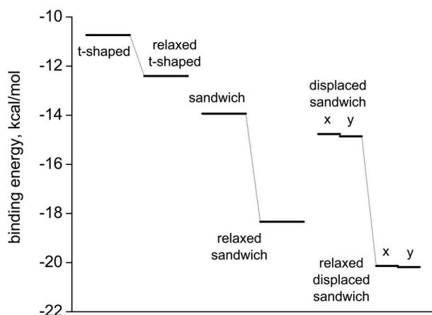
FIG. 5. Estimated binding energies of different  $(C_6H_6)_2^+$  isomers.
