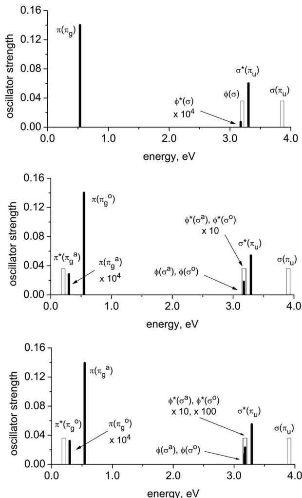
FIG. 10. Electronic states ordering and oscillator strengths of  $(C_6H_6)_2^+$  at sandwich (a) and  $x$ - and  $y$ -displaced sandwich [(b) and (c)] configurations. Empty bars denote symmetry forbidden transitions.
