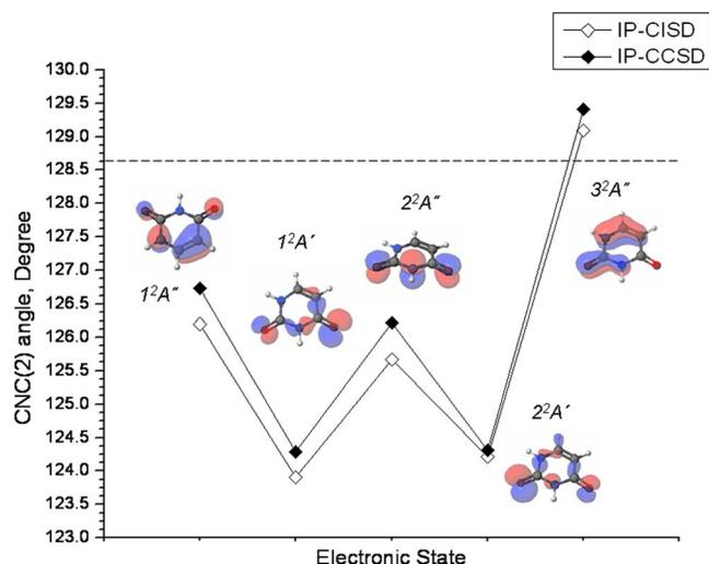
FIG. 4. (Color online) The CNC(2) angle in the five lowest electronic states of uracil cation. Dashed line shows the corresponding value at the geometry of neutral.
