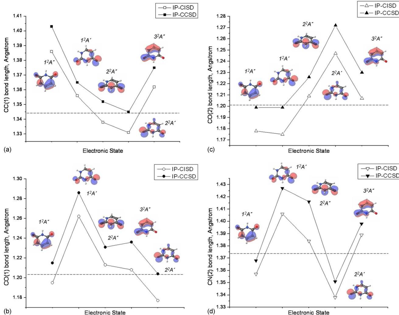
FIG. 3. (Color online) Selected bond lengths in the five lowest electronic states of the uracil cation. The corresponding values of the neutral are shown by dashed lines. The MOs from which electron is removed are shown for each state.
