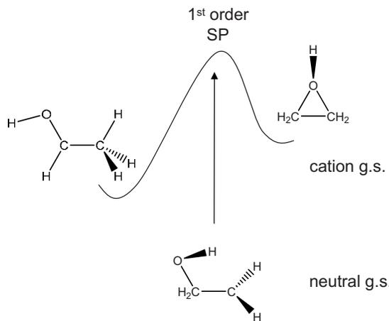
FIG. 1. First ionization of  $\text{CH}_2\text{CH}_2\text{OH}$ . On the cation PES there is a first order saddle point in the Franck–Condon region which connects the  $\text{CH}_3\text{CHOH}^+$  and  $\text{CH}_2(\text{OH})\text{CH}_2^+$  conformers. The calculated vertical and adiabatic IEs are  $\text{VIE}=8.93$  eV,  $\text{AIE}=6.21$  and  $7.37$  eV.
